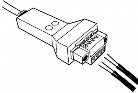
3. Use a screwdriver with a 2.5 mm wide shaft to tighten the screws above each termination point to secure the wires, using a torque of 0.196 N·m (2 kgf·cm).
