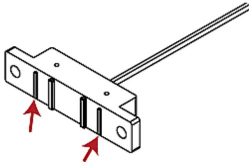
When there is some water between the two poles, it causes current loop back on the water sensor to trigger the alarm.
