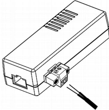
3. Use a screwdriver with a 2.5 mm wide shaft to tighten the screws above each termination point to secure the wires, using a torque of 0.196 N·m (2 kgf·cm).
