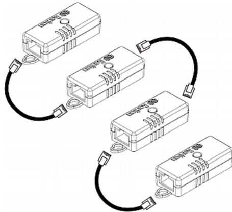
3. Make sure the total number of cascaded sensors does not exceed the maximum number of sensors supported per sensor port. See **Supported Maximum Number of Sensors and Actuators** (on page 62).
