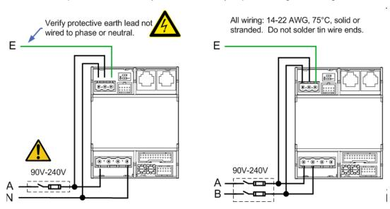
Powering from an auxiliary single phase circuit is required when the voltage measurement circuit exceeds 240V, or when continued operation is required if the voltage measurement inputs turn off.
