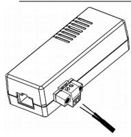
3. Use a screwdriver with a 2.5 mm wide shaft to tighten the screws above each termination point to secure the wires, using a torque of 0.196 N·m ( $2 \text{ kgf} \cdot \text{cm}$ ).
