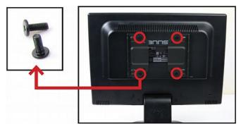
3. Align two screw holes on each side of the User Station with those on the VESA mount.
