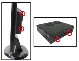
4. Tighten two sides securely using four appropriate screws.
