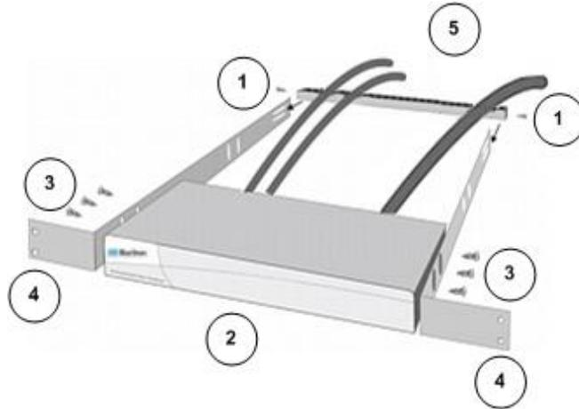
1. Secure the cable-support bar to the back end of the side brackets using two of the included screws.
