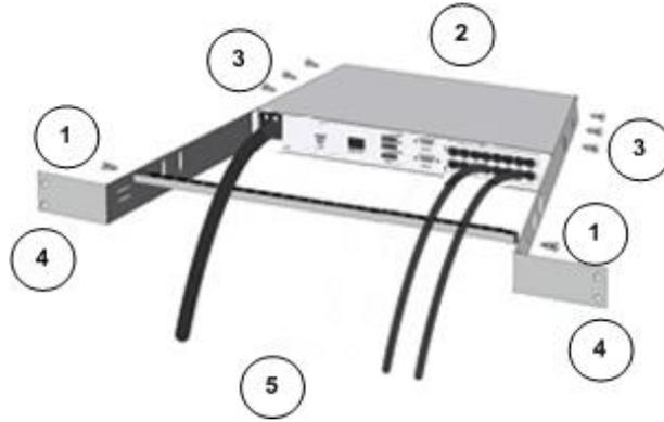
1. Secure the cable-support bar to the front end of the side brackets, near the side brackets' "ears," using two of the included screws.
