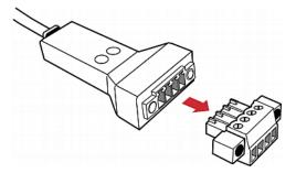
3. After connecting detectors/switches to the terminal module, plug the terminal module back into the sensor box, and then tighten the screws at two sides of the terminal module.
