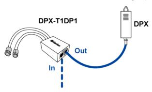
Note: You CANNOT cascade more than two sensor packages in this DPX sensor chain.
