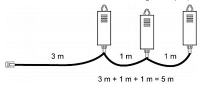
The total cabling length between the PDU/EMX/BCM and one DPX-T3H1 is 49' (15 m) as illustrated below.
