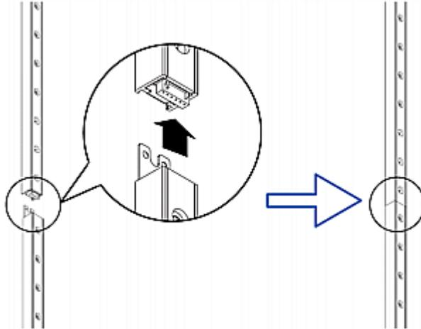
2. Connect another 8U slave strip to the one being attached to the master strip in the same manner as Step 1.
