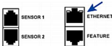
**Warning:** Accidentally plugging an RS-232 RJ-45 connector into the ETHERNET port can cause permanent damages to the Ethernet hardware.
