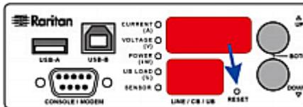
This diagram shows the location of the reset button on 2U models.
