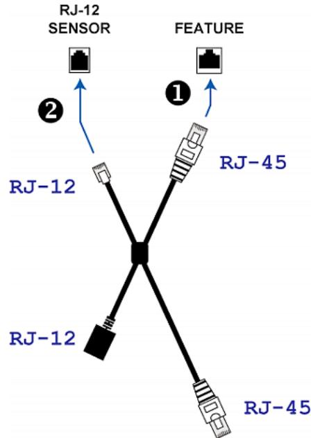
3. Plug the male RJ-45 connector at the longer end of the X cable into the RJ-45 port labeled "Input" on the composite asset strips.
