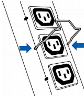
3. Plug the power cord into the outlet, and press the clip toward the power cord until it holds the cord firmly. The clip's central part holding the plug should face downwards toward the ground, like an inverted "U". This allows gravity to keep the clip in place.
