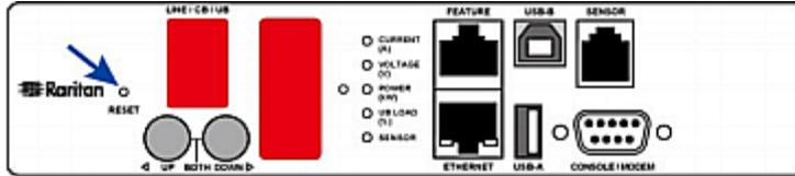
This diagram shows the location of the reset button on 1U models.
