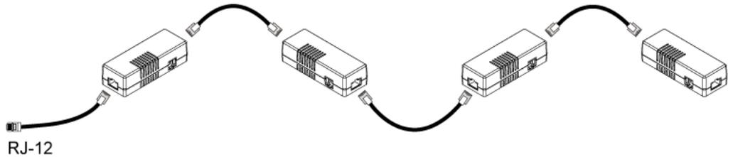
3. Connect the first DX sensor package to the PX2.
