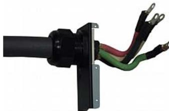
Temporarily hand tighten the gland nut and verify the cord cannot be twisted or pushed or pulled in the gland. Do not proceed if hand tightening results in a loose cord. In some models, especially in-line monitors, the flexible cord's diameter may be too small for the cable gland. A sealing ring for smaller diameter line cords may have been included with the Raritan product, or can be requested from Raritan, to reduce the inside diameter of the cable gland.
