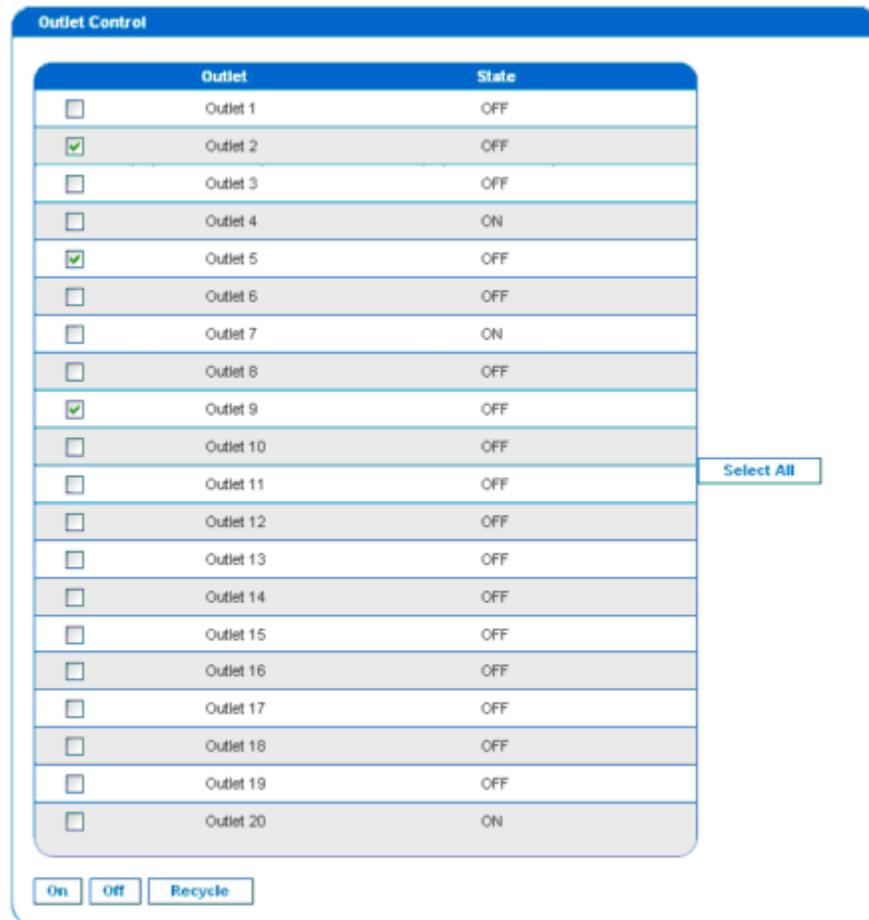
2. Check the box of outlet number you wish to control, and click On/Off buttons to power on/off the selected outlet(s).
