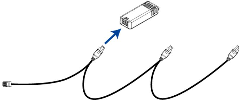
2. Connect remaining DPX2 sensor packages to the second and then the third head connector.
