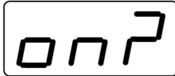
3. Press and hold the Up button until the above confirmation message disappears, indicating that the outlet has been turned on.
