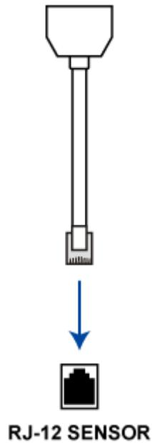
2. The cable has two RJ-12 sensor ports. Connect DPX sensor packages to the cable's sensor ports.
