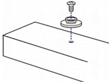
4. Screw a button in the screw hole near the top. The recommended torque for the button is 1.96 N·m (20 kgf·cm).
