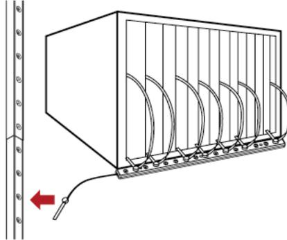
6. Repeat the above steps to connect additional blade extension strips. Up to 128 asset tags on blade extension strips are supported per FEATURE port.
