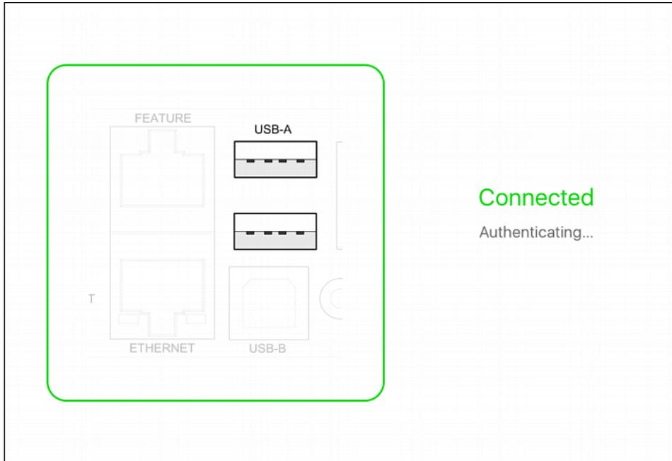
2. If the factory-default user credentials "admin/raritan" remain unchanged, PDView automatically logs in to the PX2 web interface. If they have been changed, the login screen displays instead and you must enter appropriate user credentials for login.
