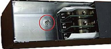
For in-line monitors, make sure to identify the inlet terminal blocks (rear of monitor) and outlet terminal blocks (front of monitor). Each inlet terminal block has a corresponding outlet terminal block.
