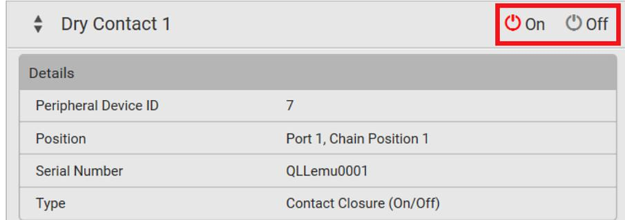
The screenshot shows a control panel for 'Dry Contact 1'. At the top right, there are two buttons: 'On' (with a red power icon) and 'Off' (with a grey power icon). The 'On' button is highlighted with a red rectangular box. Below the buttons is a 'Details' table:
