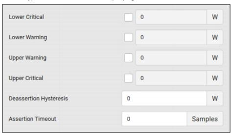
For concepts of thresholds, deassertion hysteresis and assertion timeout, see Sensor Threshold Settings (on page 802).
