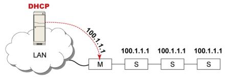
In this mode, the DHCP server communicates with the master device alone and assigns one IP address to the master device. All slave devices share the same IP address as the master device.
