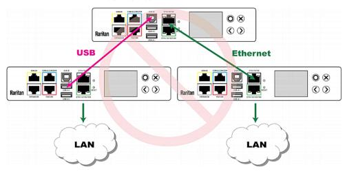
• One cascaded device has two downstream devices.
