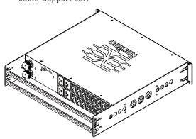
5. Fasten the rackmount brackets' ears to the rack using your own fasteners.
