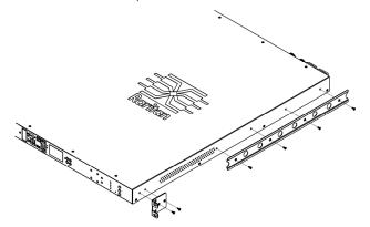
2. Adjust slide-rail assemblies to match your rack posts and fasten them to the rack using your own fasteners.
