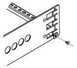
4. On a 2U model, repeat the above steps to install another cable-support bar.
