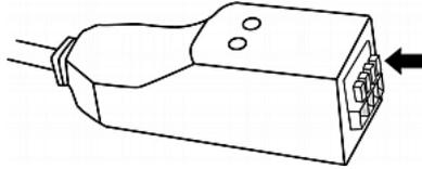
3. Fully insert each wire of both detectors/switches into each termination point.
