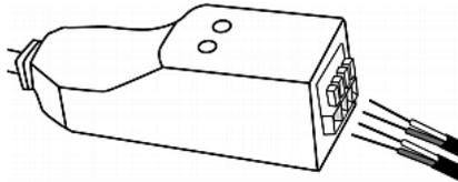
4. Release the tiny rectangular buttons after inserting the wires properly.
