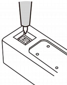
5. To set the Normal state for channel 2, repeat Step 4 for adjusting the other dip switch's setting.
