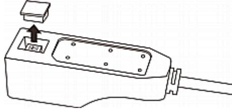
3. To set the Normal state for channel 1, locate the dip switch labeled 1.
