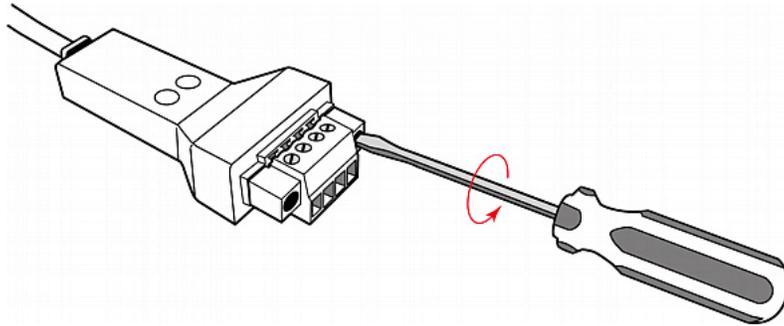
2. Separate the terminal module from the sensor box.
