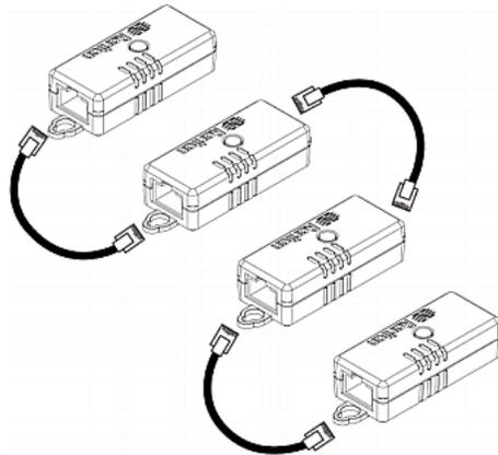
3. Make sure the total number of cascaded sensors does not exceed the maximum number of sensors supported per sensor port. See ***Supported Maximum Number of Sensors and Actuators*** (on page 66).
