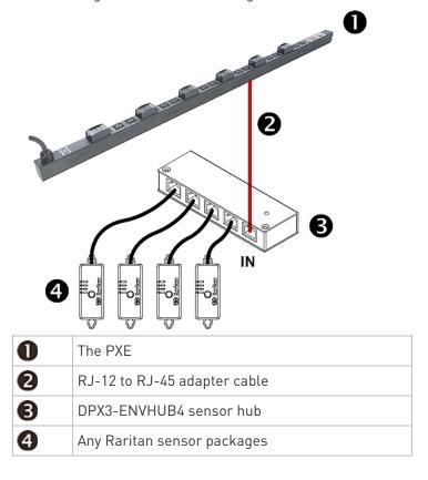
This diagram illustrates a configuration with a sensor hub connected.
