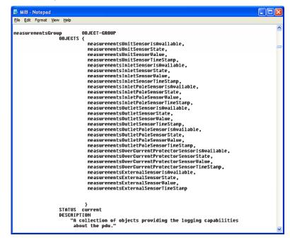
For example, the measurementsGroup group contains objects for sensor readings of PXE as a whole. One object listed under this group, measurementsUnitSensorValue, is described later in the MIB as "The sensor value". pduRatedCurrent, part of the configGroup group, describes the PDU current rating.
