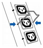
3. Plug the power cord into the outlet, and press the clip toward the power cord until it holds the cord firmly. The clip's central part holding the plug should face downwards toward the ground, like an inverted "U". This allows gravity to keep the clip in place.
