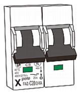
3. Examine your PXE and the connected equipment to remove or resolve the cause that results in the overload or short circuit. This step is required, or you cannot proceed with the next step.
