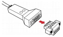
3. After connecting detectors/switches to the terminal module, plug the terminal module back into the sensor box, and then tighten the screws at two sides of the terminal module.
