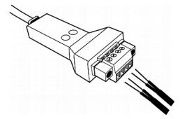
Use a screwdriver with a 2.5 mm wide shaft to tighten the screws above each termination point to secure the wires, using a torque of 0.196 N·m (2 kgf·cm).
