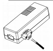
Use a screwdriver with a 2.5 mm wide shaft to tighten the screws above each termination point to secure the wires, using a torque of 0.196 N⋅m (2 kgf⋅cm).
