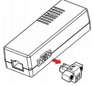
3. After connecting detectors/switches to the terminal module, plug the terminal module back into the sensor box, and then tighten the screws at two sides of the terminal module.
