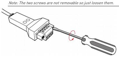
2. Separate the terminal module from the sensor box.
