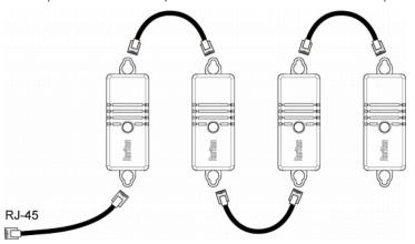
3. Make sure the total number of cascaded sensors does not exceed 32 per sensor port. See *Supported Maximum Number of Sensors and Actuators* (on page 77).
