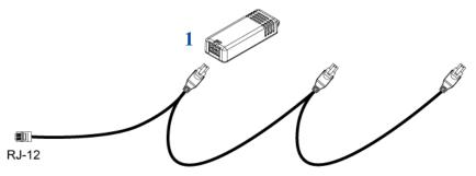
• Scenario B: When only two sensors are connected, always connect them to the first two head connectors.
